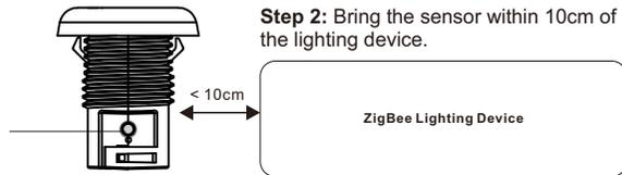
**Step 2:** Bring the sensor within 10cm of the lighting device.
