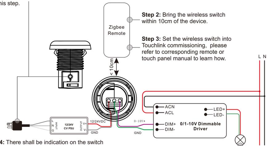
**Step 4:** There shall be indication on the switch for successful link and connected light will flash twice.
