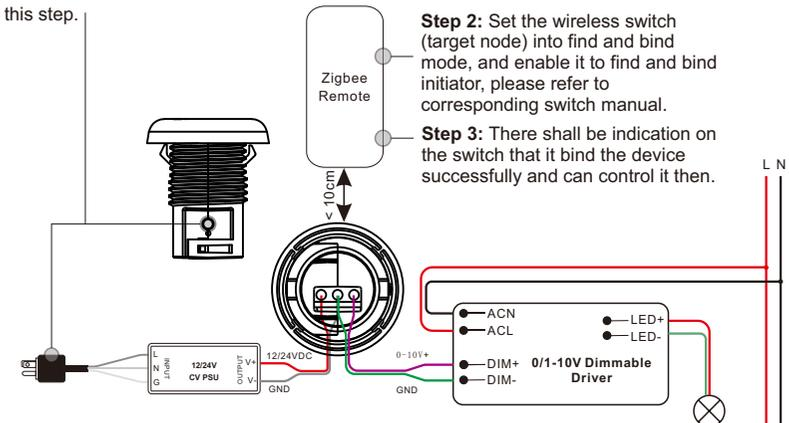
**Step 2:** Set the wireless switch (target node) into find and bind mode, and enable it to find and bind initiator, please refer to corresponding switch manual.
