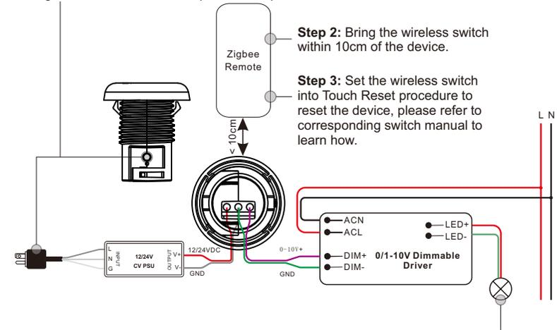
**Step 2:** Bring the wireless switch within 10cm of the device.
