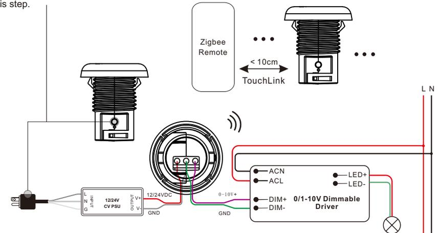
**Step 2:** Set another light device or wireless switch into network pairing mode and pair to the network, refer to their manuals.
